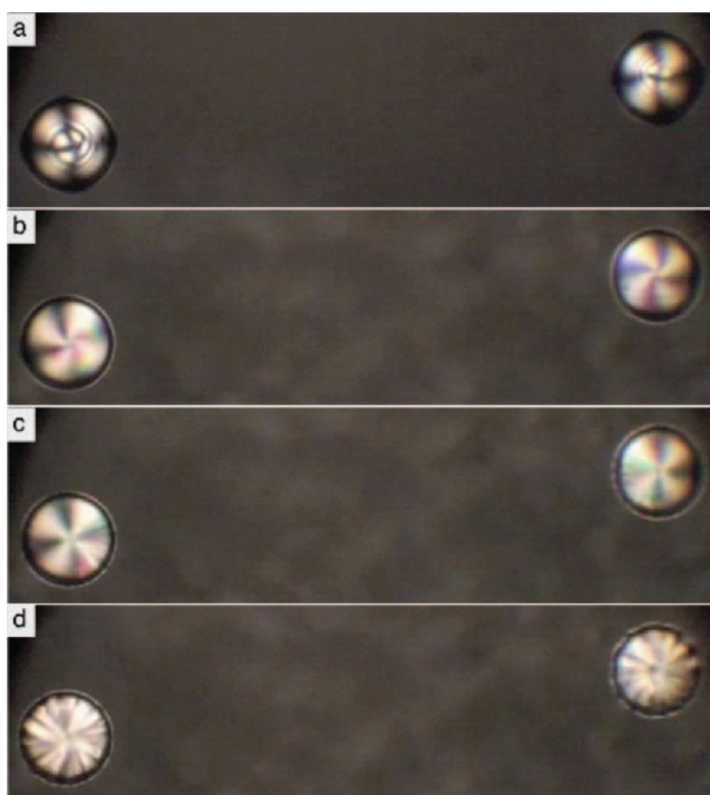
Figure 6. Two shells going through the same transition as in Fig. 5. Note how the twist is in opposite directions in the two shells.
